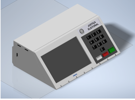
Figure 4: 3D final model of the voter terminal
