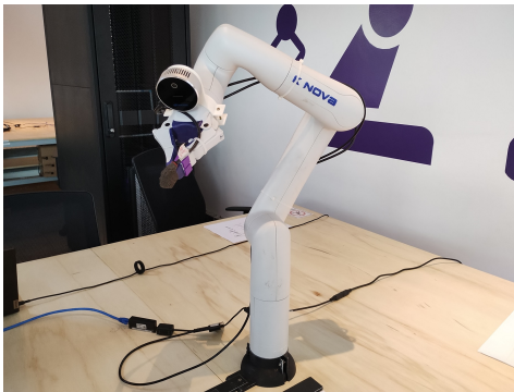
Figure 6: Robot Kinova gen3 lite used to capture the dataset with support and camera
