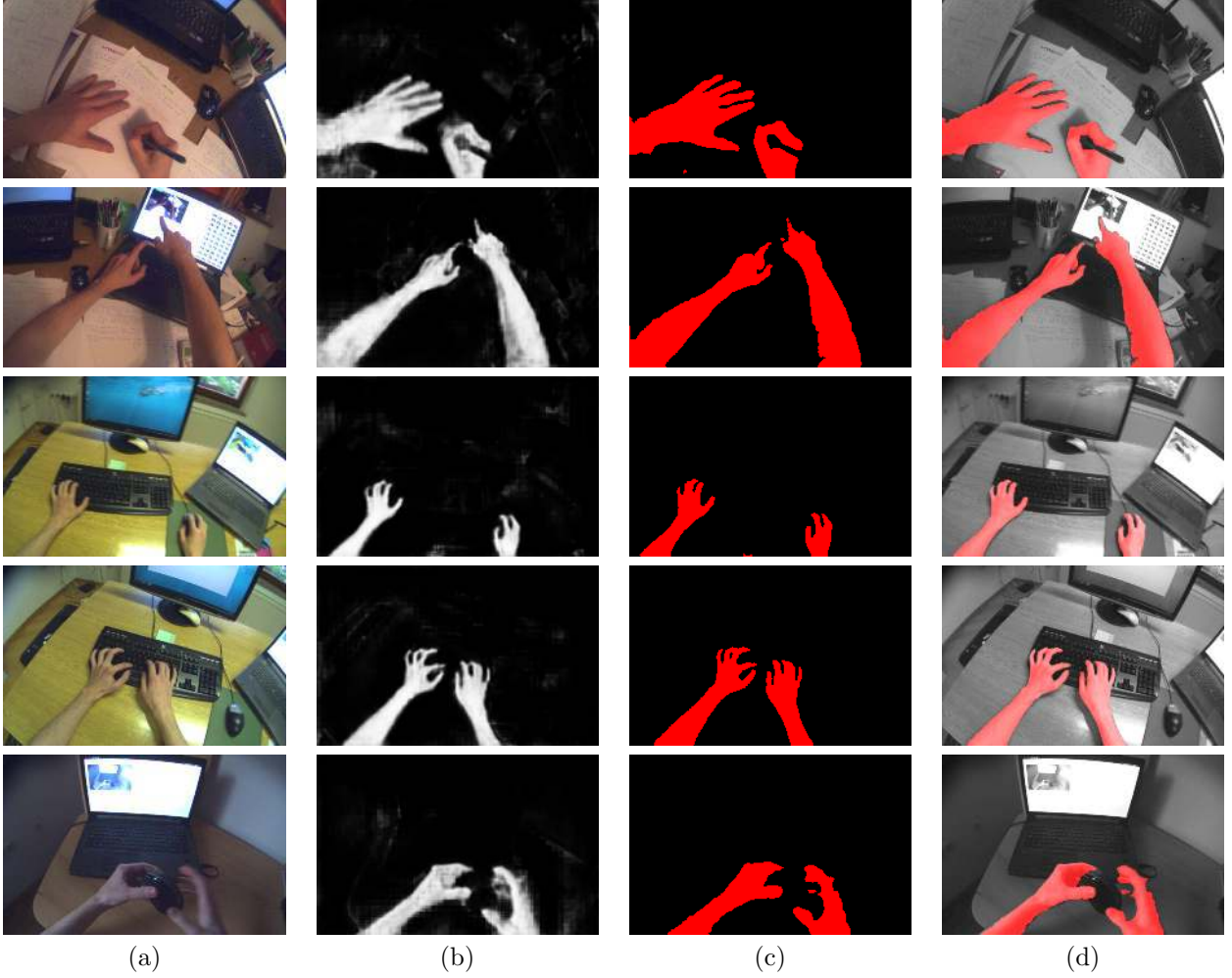
Figure 9: Images and their segmentations. (a) Original image; (b) Upscaled segmentation predicted by the first part of our network; (c) Final segmentation; (d) composition of the final segmentation into the original image.
