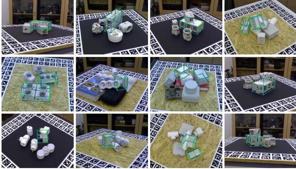
Fig. 8. Qualitative results on the unknown objects of the test scenes from T-LESS. Green bounding boxes denote ground truth poses, blue bounding boxes correspond to our predicted poses.
