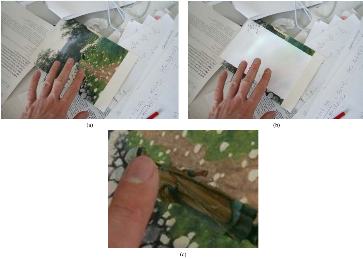
Figure 4: Handling a large occlusion. (a) The postcard of Fig. 1 is occluded by several fingers. (b) The diminished reality version of the postcard. (c) A detail of the augmented postcard. The visibility map is computed accurately enough so that rendering the virtual character under the finger appears realistic.
