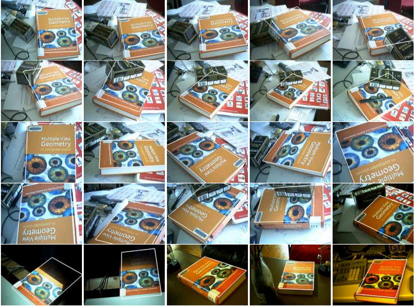
Figure 1: The book is detected and its 3D pose estimated at 25Hz, on a standard PC, in spite of partial occlusion, cluttered background, and large illumination and pose changes.
