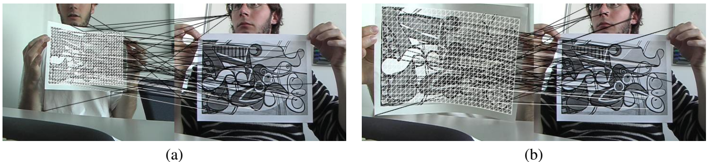
Fig. 19. Detecting a deforming sheet of paper at 10Hz on a 2.8 GHz PC. (a) The left image is the input image in which the sheet of paper is detected and its deformation estimated. The right one is the training image. The lines represent the matches recovered using our method. Black ones correspond to those estimated to be outliers and the white ones to inliers. (b) Same thing for a different input image.
