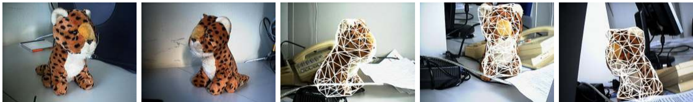
Fig. 2. The method is just as effective for 3-D objects. In this experiment, we detected the stuffed tiger in the three images to the right using a 3-D model reconstructed from several views such as the two first images on the left. Note that it reprojects at the right place in all three images.
