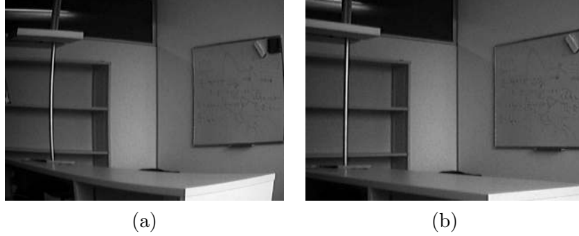
Fig. 2.3 Undistorting an image. (a) Due to perspective distortion, projections of straight lines are curved. (b) In the undistorted image, the projections of straight lines are now straight.
