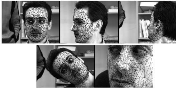
Fig. 4.6 Face tracking using interest points and one reference image shown on the top left. (From [137].)
