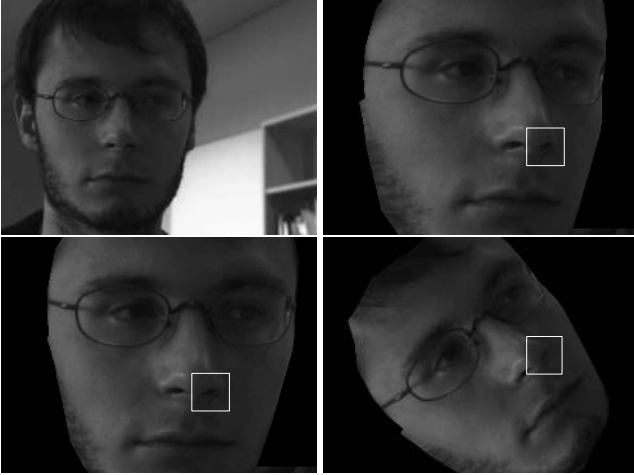
Figure 3: Three synthetic views of a human face, generated from the original image on the top left. The patches extracted from these images to build a viewset of a keypoint on the nose are represented.
