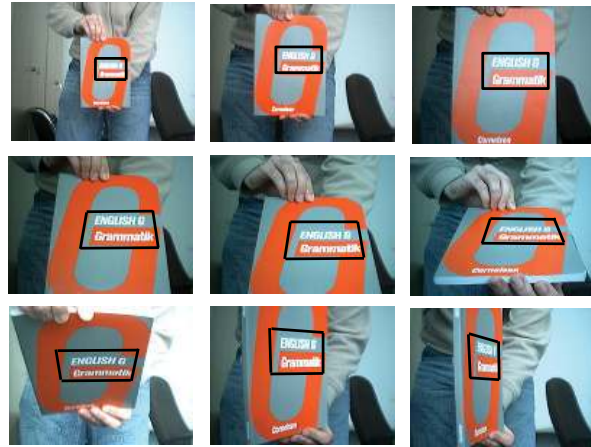
Fig. 17 Training framework. We incrementally train the classifiers and the linear predictors over the frames of a training sequence. To this end, the object is automatically registered in each incoming frame using the current state of these classifiers and linear predictors.
