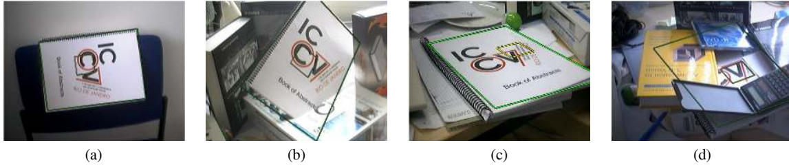
Fig. 19 Accuracy of ALGO1 of the retrieved transformation. For each of these images, we draw the borders of the book estimated from a single patch. This is made possible by the fact we estimate a full perspective transform instead of only an affine one.
