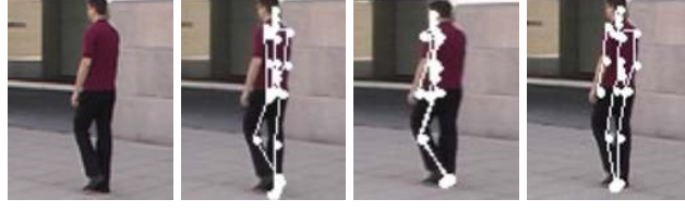
Figure 3. Refinement process. The images are from left to right the input image, the initialization given by the interpolation process, the result obtained without using a background image, and finally the result obtained as proposed. Whole parts of the body can be missed when the background is not exploited.
