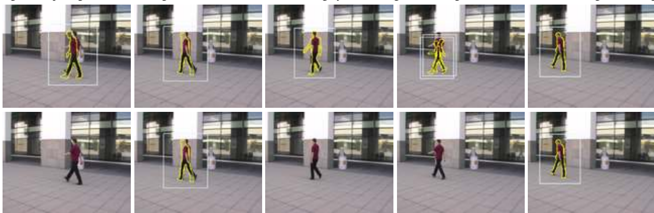
Figure 5. Filtering silhouettes with temporal consistency on an outdoor sequence acquired by a moving camera. First row: Detection hypotheses. Second row: Detections after filtering out the detection hypotheses that do not lie on the recovered most probable trajectory.
