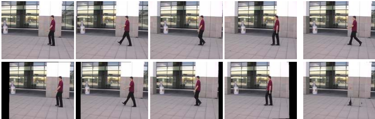
Figure 4. Synthesizing a background image. First row: The rightmost image is the reference image whose background we want to synthesize. The other 4 are those before and after it in the sequence. Second row: The same four images warped to match the reference image. Computing the median image of these and the reference image yields the rightmost image, which is the desired background image.
